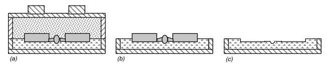
**Figure 8.** (a) The mold was rolled over and (b) the drag lifted off. (c) The finished composition match. After the sand composition has hardened the new composition match is ready for use. Note Figure 8(c) is identical to Figure 1(a).
