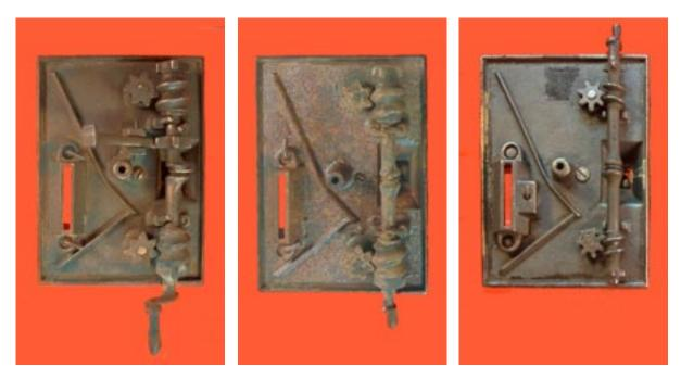
**Illustration 21.** Three different internal mechanisms used in the "Organ Bank, Cat and Dog" banks by Kyser & Rex Co.
