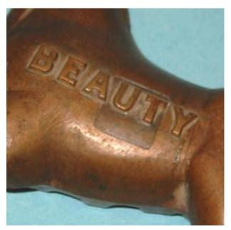
**Photo 3.** Close-up of the left side of the pattern. Notice that the square area in the center of the photo where a plug fills what was a depression for a square nut. Solder can be seen around the letters, which were applied to the pattern.
